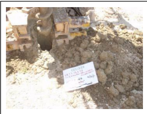
Photo 13. Arisings from SB06B (0.0m – 5.5m bgl)
